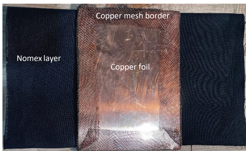
Figure 3. Liquid hydrogen refuelling barrier prototype mock-up with Nomex® base layer, copper plate, and copper mesh border.
