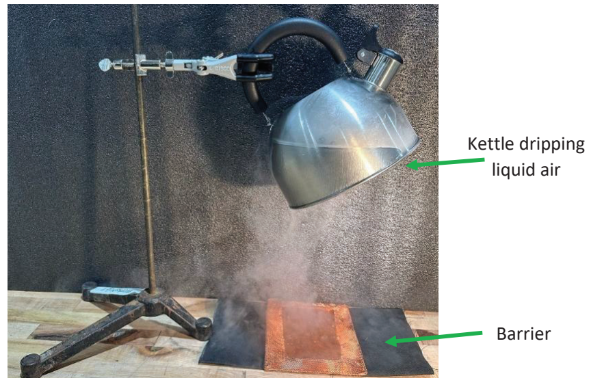
Figure 4. Experimental verification setup of mock-up liquid hydrogen refuelling barrier using liquid nitrogen in a teakettle to create liquid air.
